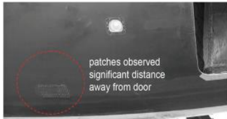
Figure 5. Example of Patch Repair [29]
