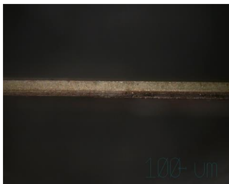
Figure 4.2. 532 nm, “1” cut of the PVDF specimen
