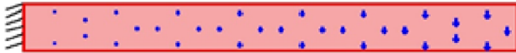
Figure 2.9. Computational scheme of the shape optimization problem of the active element of the energy harvester: initial shape, boundary condition, distributed spatial load;
