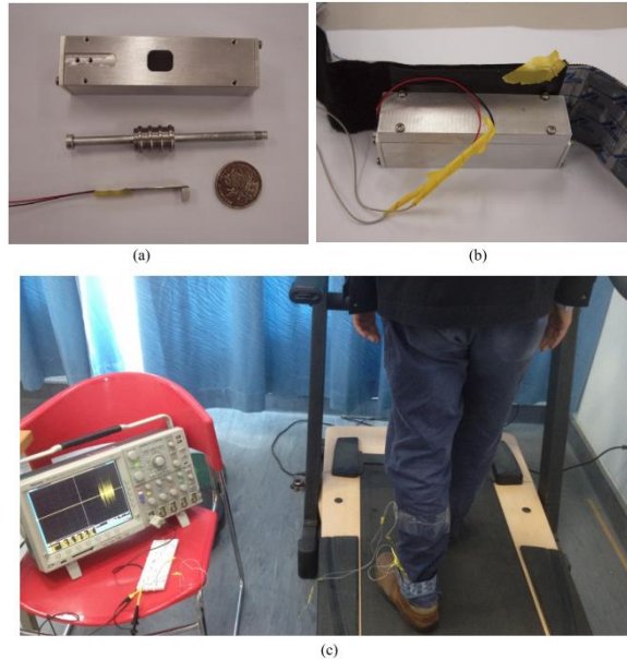
Figure 1.27. (a) Photograph of the actual prototype, showing the PZT bimorph, shaft, cylinder, cover and frame. (b) Assembled prototype
