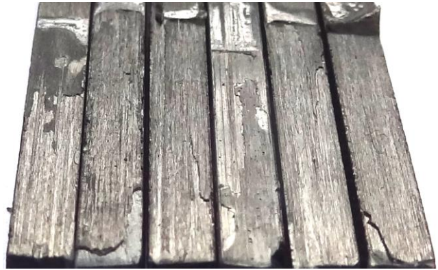
Fig. 6 Views of adhesion zones after fatigue fracture
