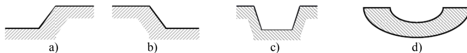
Fig. 1. Possible defects of the road: a) step up; b) step down; c) step down and up; d) bending down [6]
