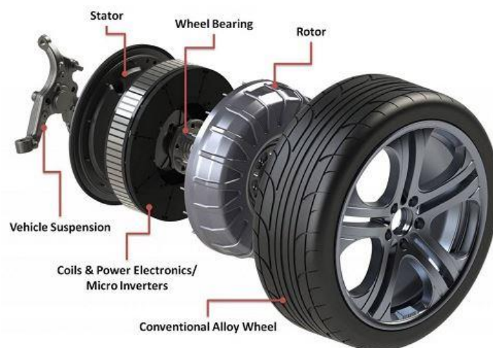
Figure 26. Basic construction of motor to wheel as powertrain [26]
