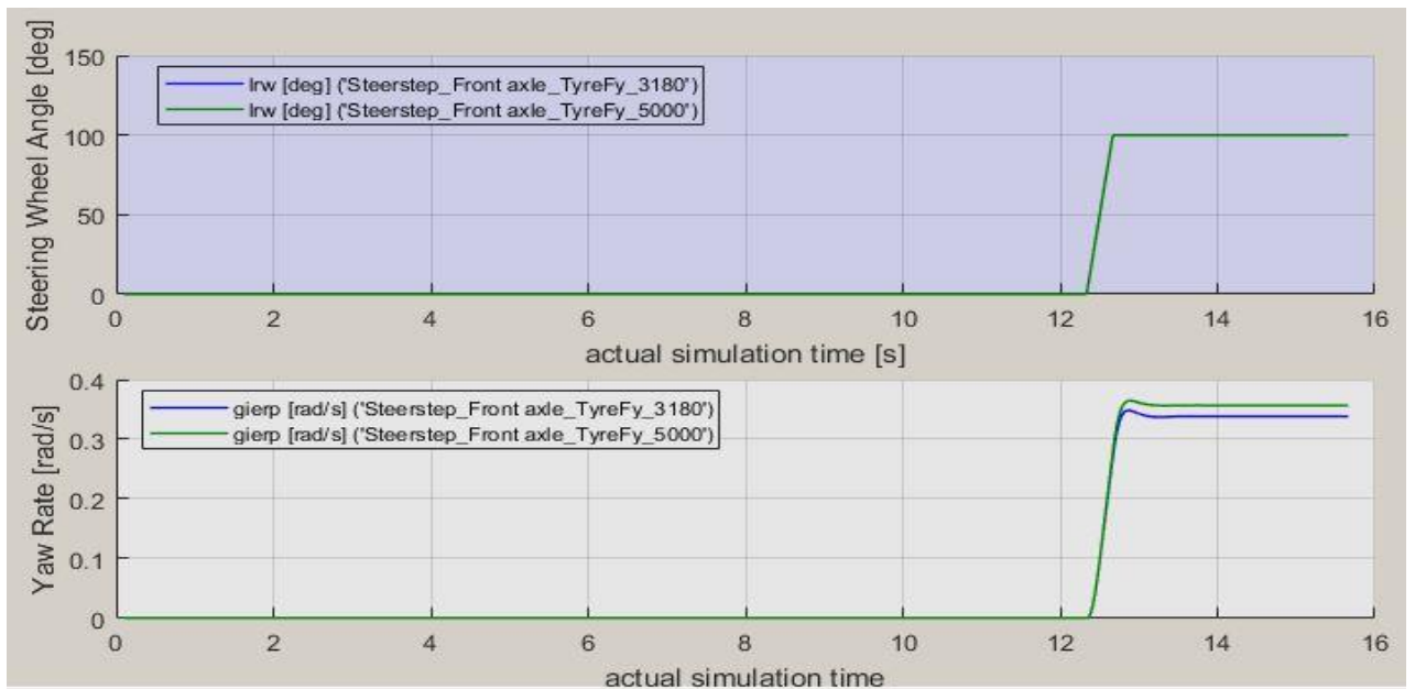
Figure 20. Steerstep yaw rate response due to steering wheel input graph
