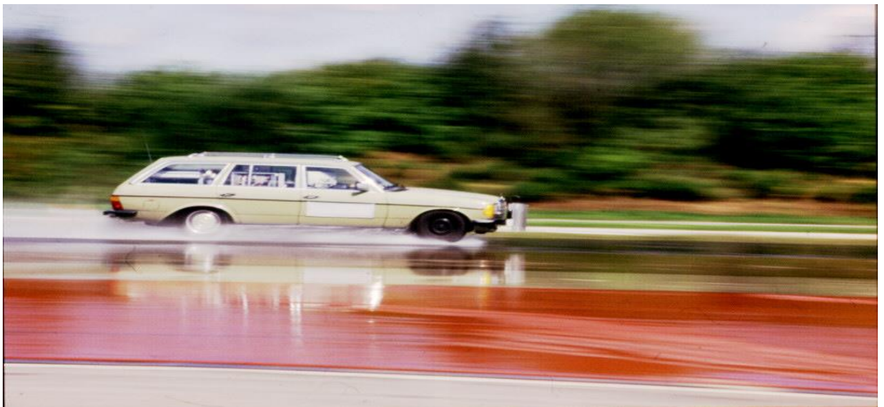
Figure 2. Testing ESP prototypes in a 1983 Mercedes-Benz 230 TE on Bosch ground [11]
