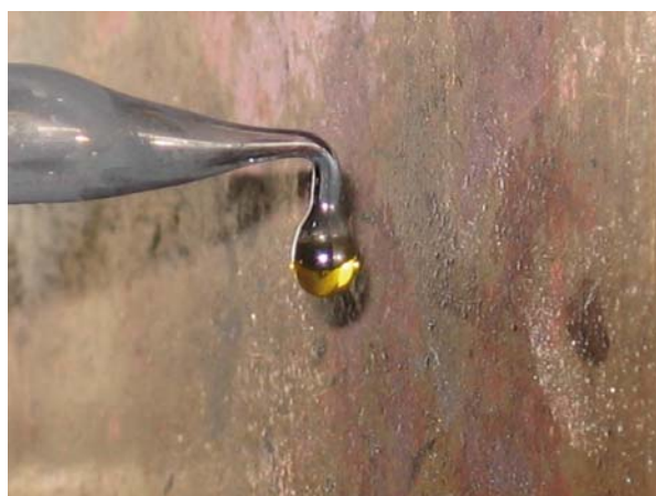
Fig. 2. Fuel droplet hanging on the suspension device
