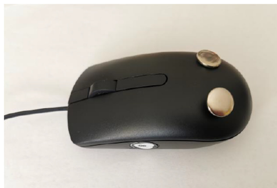
Figure 1. The developed smart mouse with PPG and GSR sensors [12].
