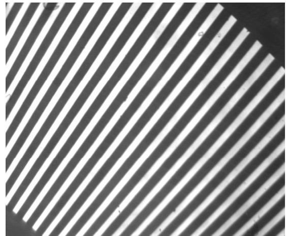
Fig. 5. Optical microscope view (light transmission mode) of the fabricated by imprint lithography angular encoder (length of lines is 0.75 \text{ mm} , scale pitch in the center of lines is 20 \mu\text{m} )
