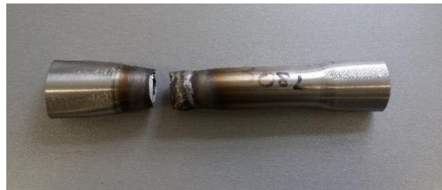
Fig. 5 Specimen after the tensile test
