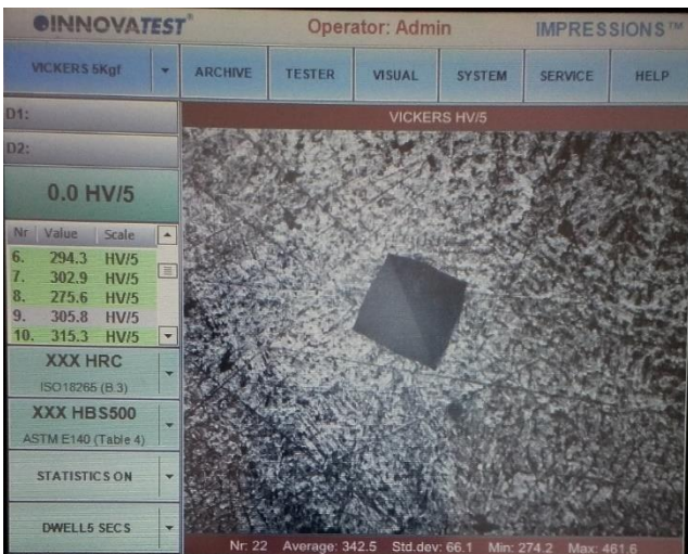
Fig. 7 Vickers hardness test result on the screen
