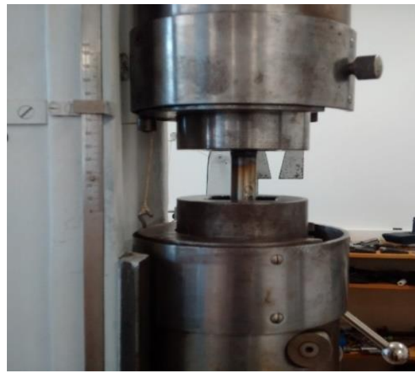
Fig. 4 The specimen fixed in the tension-compression testing machine
