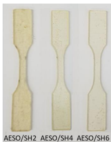
Figure 6. Images of the dog-bone shaped samples die cut from polymer samples.
