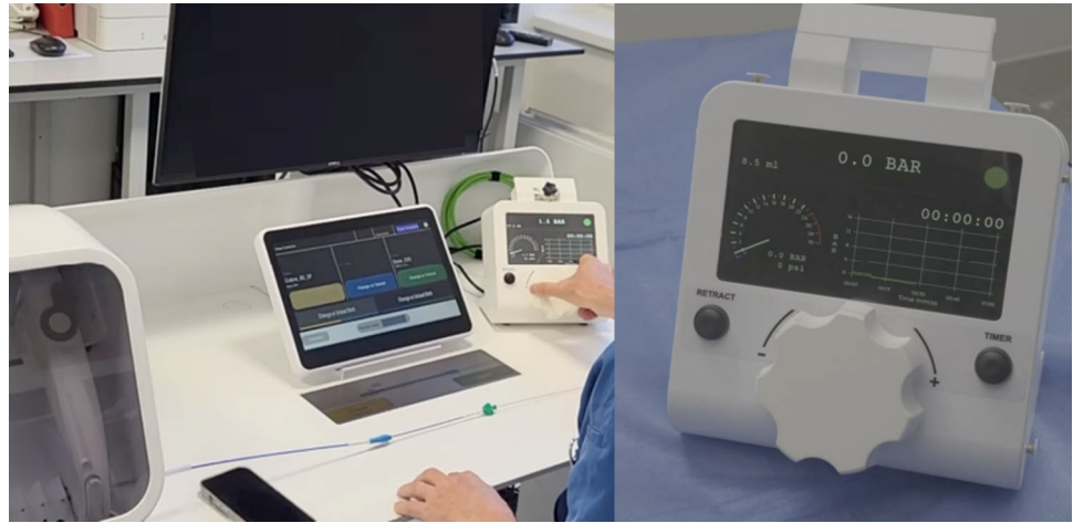
Fig. 3 The remote workstation of the SENTANTE is equipped with a system (INFLATE) that allows for remote initiation of balloon inflation or contrast injection by the bedside unit
