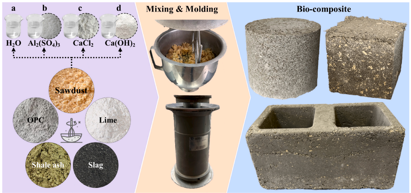
Fig. 2. Schematic overview of the bio-composite fabrication process, including sawdust pre-treatment, binder preparation, mixing, and molding procedures.
