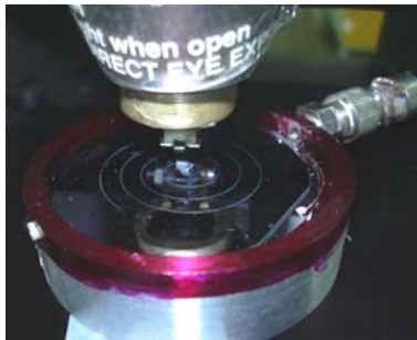
Fig. 9 Experimental setup for AFM investigations
