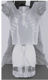
Fig. 1. An anthropomorphic phantom “Lungman”
