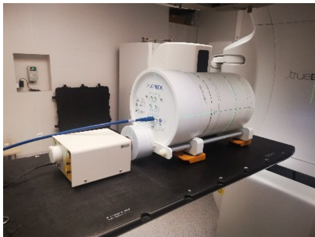
Fig. 2. ArcCheck array setup before performing dose measurements.
