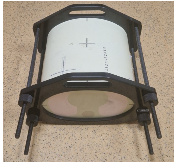
Fig. 1. CIRS 002LFC anthropomorphic chest phantom.
