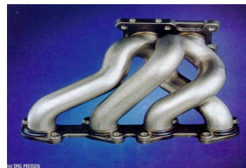
Fig. 2 Part, manufactured by hydroforming [1]
