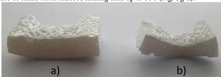
Fig. 6. An optical images of expanded polystyrene with (a) and without (b) SiO 2 film after 60 s of flame torch induced heat experiment
