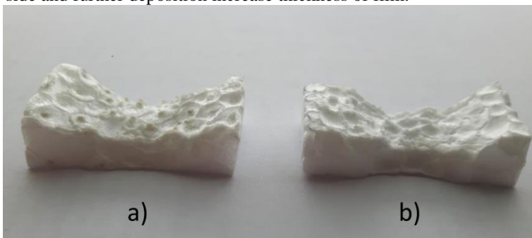
Fig. 11. An optical images of expanded polystyrene with (a) and without (b) SiO 2 fractures incorporated into the bulk after 40 s of flame torch induced heat experiment
