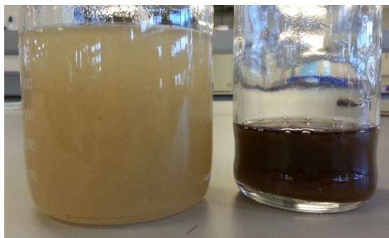
Figure 3.15. Photos of the biomass suspension used to inoculate three lab-scale BAC reactors (right) and the biomass suspension obtained from R2 at the end of the reactor runs (left)
