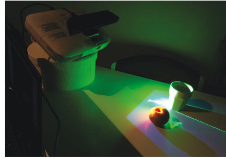
FIGURE 1: Example scene showing object selection UI that is shown to the user with camera-projector system. The system performs automatic projection mapping using depth camera information.
