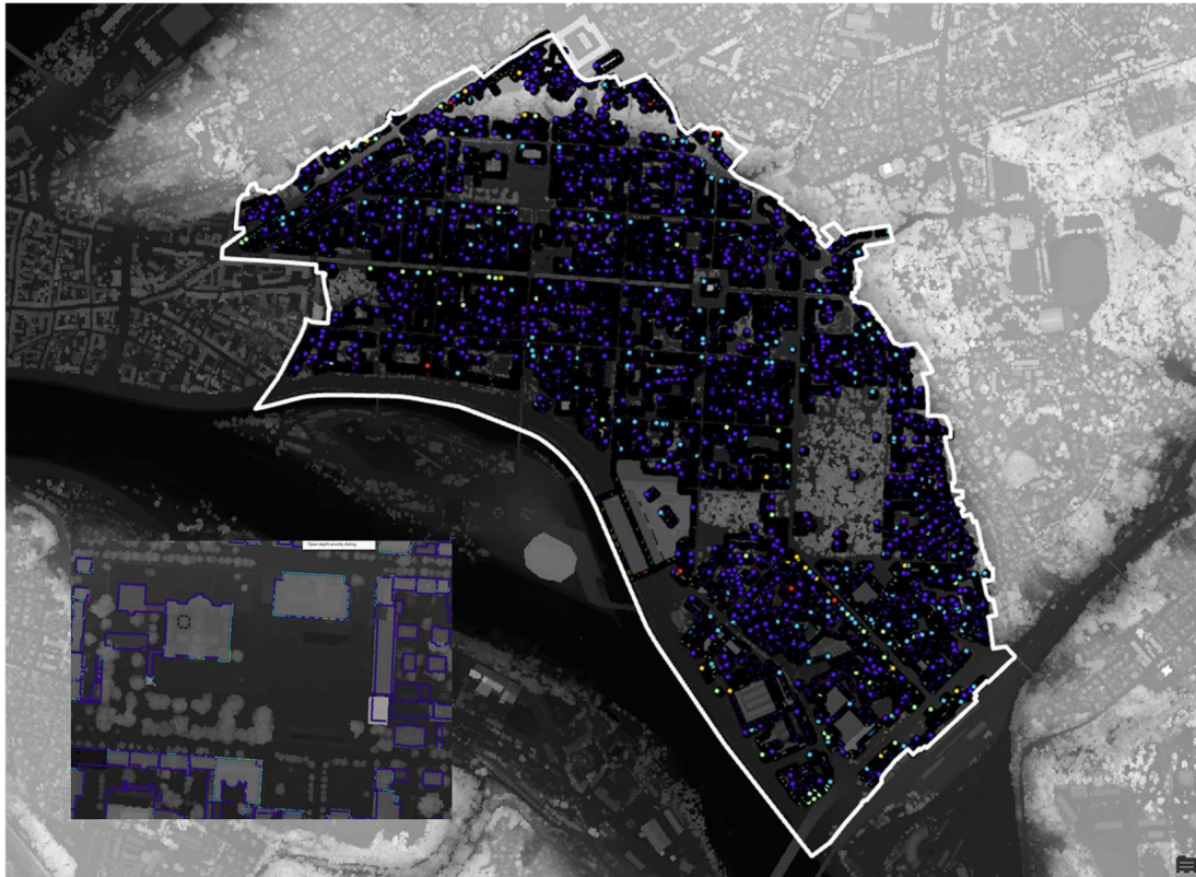
Figure A5. Visibility is the number of points from which each point of the facade is visible based on spatial join analysis of GIS. Viewshed analysis was made on both rasters: with trees and without trees.
