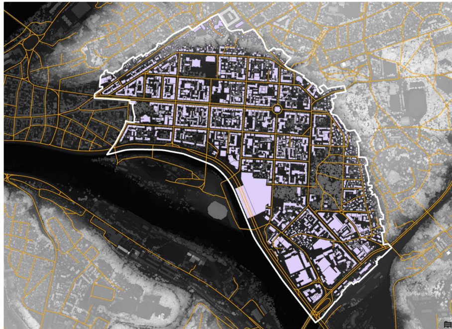
Figure A1. Raster surface data with building polygons and walking paths and streets added. White line represents the boundary of the investigated area.
