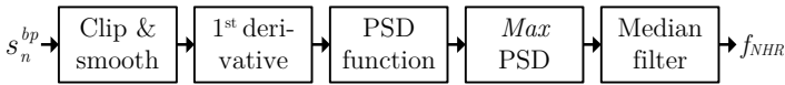
Fig. 4.8. Block diagram of the normal heart rate estimator. Here, s_k^{bp} is a 12 s segment of the preprocessed PPG.
