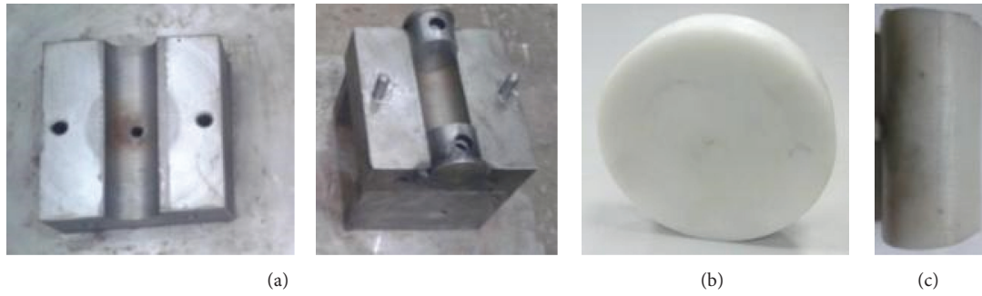
FIGURE 1: Injection die and products. (a) Photograph view of short-rod injection die. (b) Product acetal flange. (c) Product acetal short rods.
