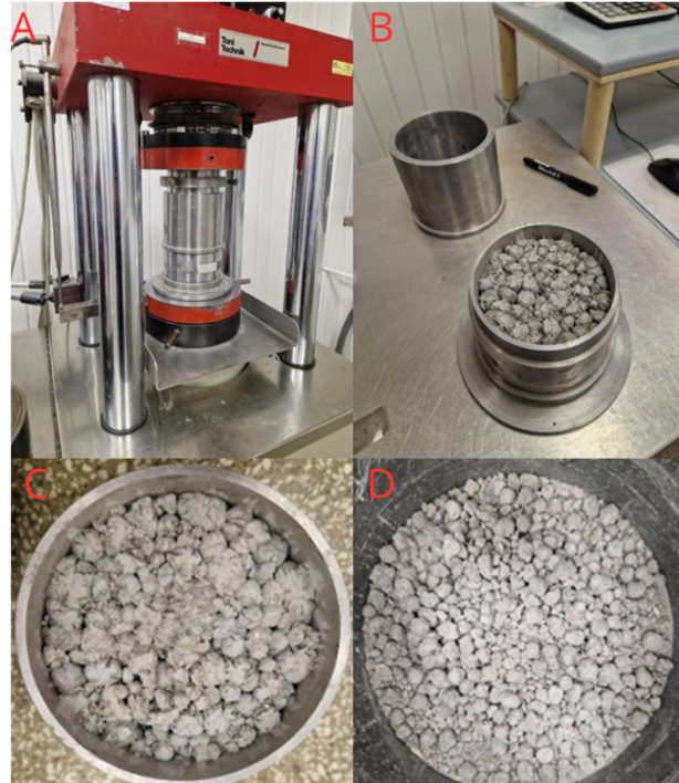
Figure 3. (A) Hydraulic press, (B) pressing cylinder, (C) samples in the crushing cylinder, and (D) crushed aggregates removed from cylinder.
