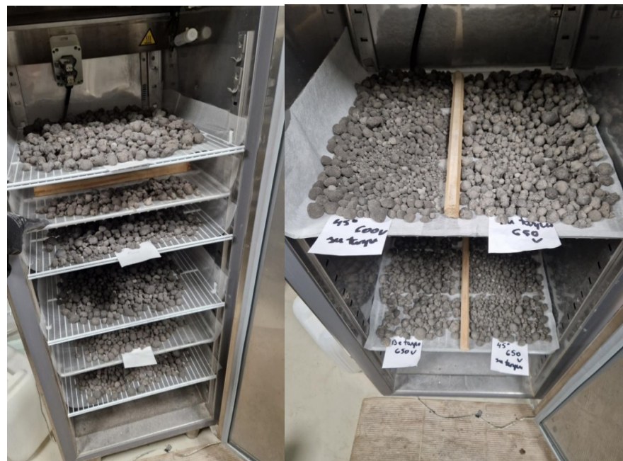
Figure 2. Carbonization of aggregates in a special chamber.
