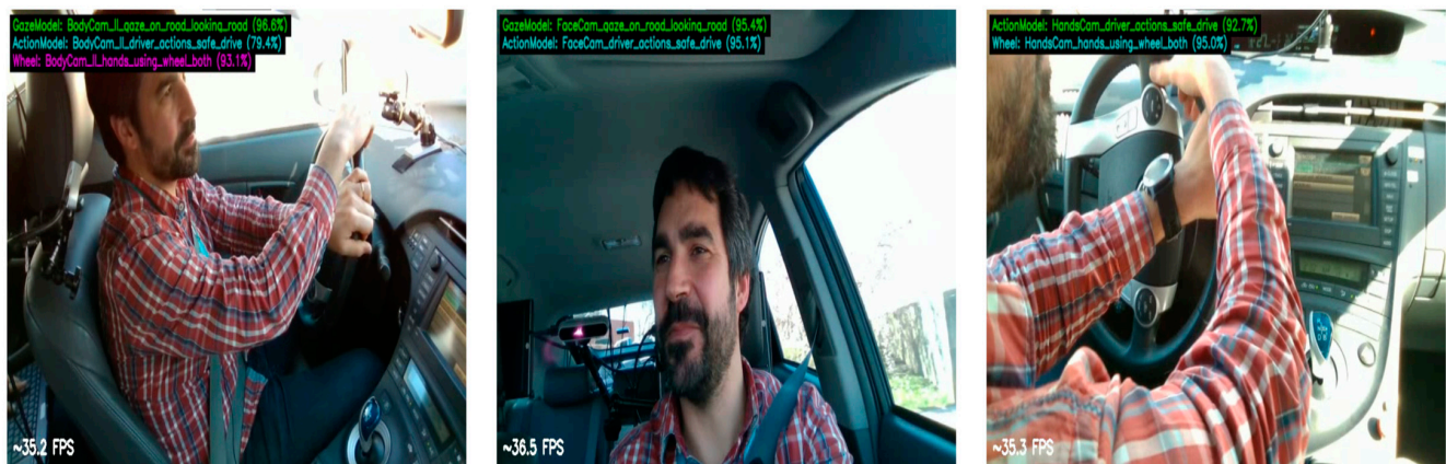
Figure 7. Example of testing outputs for multi-perspective, multi-task model at the same time point from testing videos from different perspectives.
