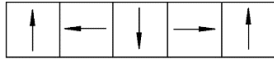
Fig. 1 General representation of permanent magnets arranged in Halbach array for one wavelength
