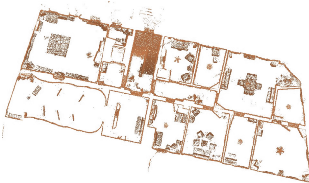
Fig. 1. The visible floor plan outline of the analyzed building from laser scanning [authors' image].
