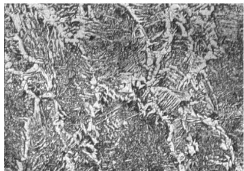
Fig. 5. Microstructure of layer of A2 alloy (×150)
