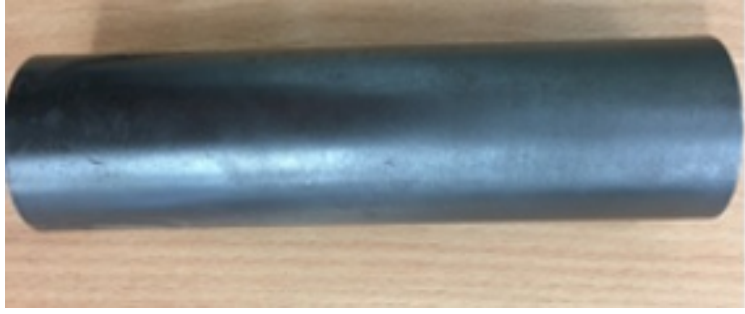
Figure 9.3 Workpiece for the orthogonal cutting process
