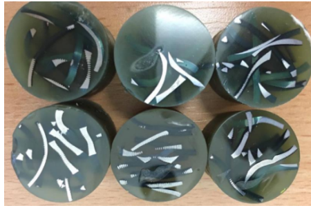
Figure 16.2 Cubes after polishing. In this figure, the chips are clearly visible after DIAMANT polishing
