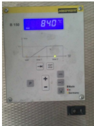
Figure 10.2 Heating Treatment Temperature
