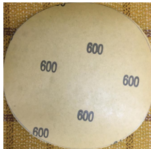
Figure 16.3 P600 AUTO-PAPER (emery paper) for the 1st operation of the grinding process
