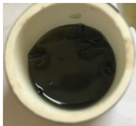
Figure 16.1 PVC pipe with the length of 3-4cm and open in one side of the pipe
