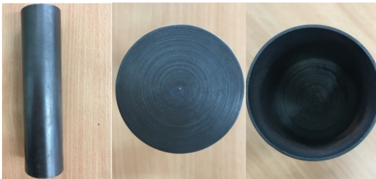
Figure 10.1 Steel S355JRG3 before the cutting process of orthogonal turning process
