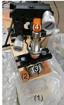
Fig. 3.21 Vibrating motors (3) on the cantilever (2) with damping element (1) and displacement sensor (4) on the top
