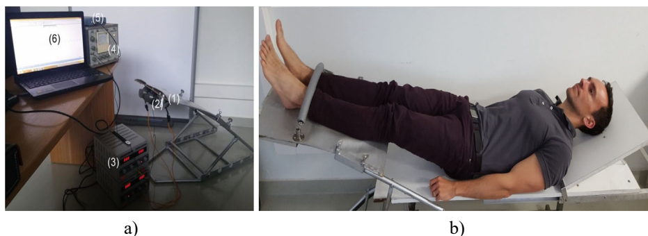
Fig. 3.53 a Experimental set-up for legs actuation: 1—legs actuator with motors and unbalanced masses; 2—acceleration sensor KB12; 3—power suppliers (0-30 V/20A, adjustable); 4—Robotron 00,032; 5—Pico scope 3424; 6—PC with Pico scope 6 software; b simulation of therapy with experimental set-up
