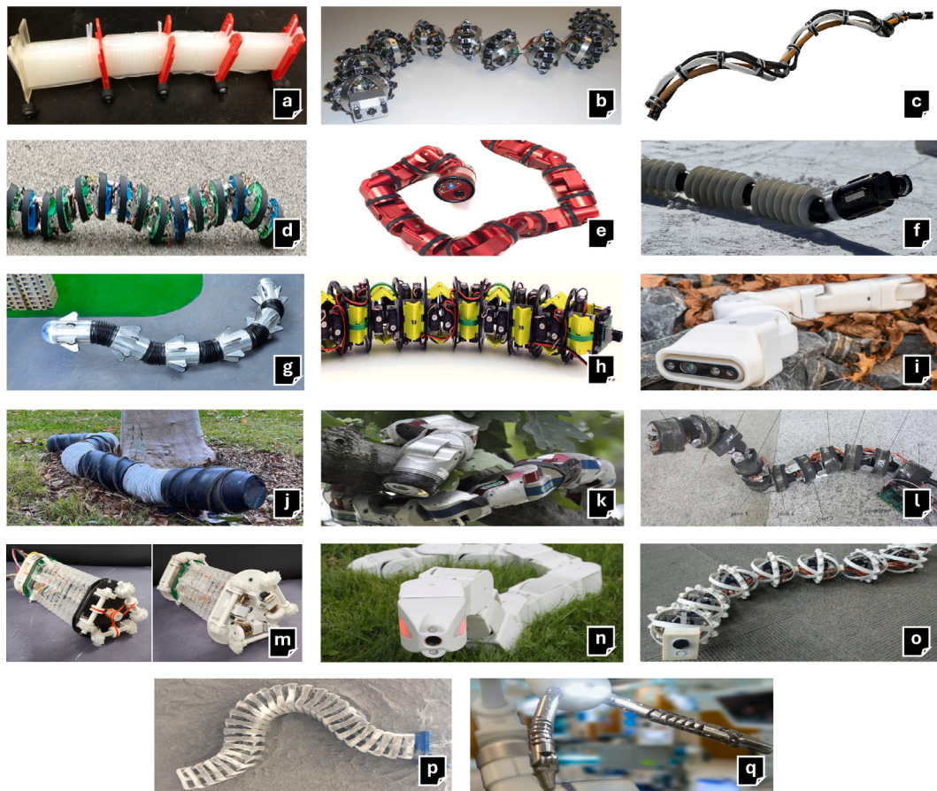
Fig. 4. Snake robots in literature navigating diverse terrains, showcasing adaptability and locomotion on uneven and challenging surfaces: (a) [54] (b) [55] (c) [56] (d) [57] (e) [58] (f) [59] (g) [60] (h) [61] (i) [10] (j) [62] (k) [63] (l) [64] (m) [65] (n) [66] (o) [67] (p) [68] (q) [53].
