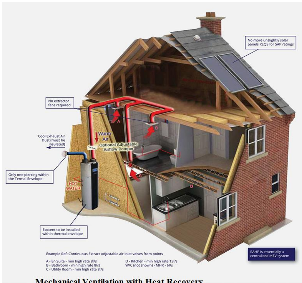
19.fig: Mechanical ventilation with heat recovery system [55]
