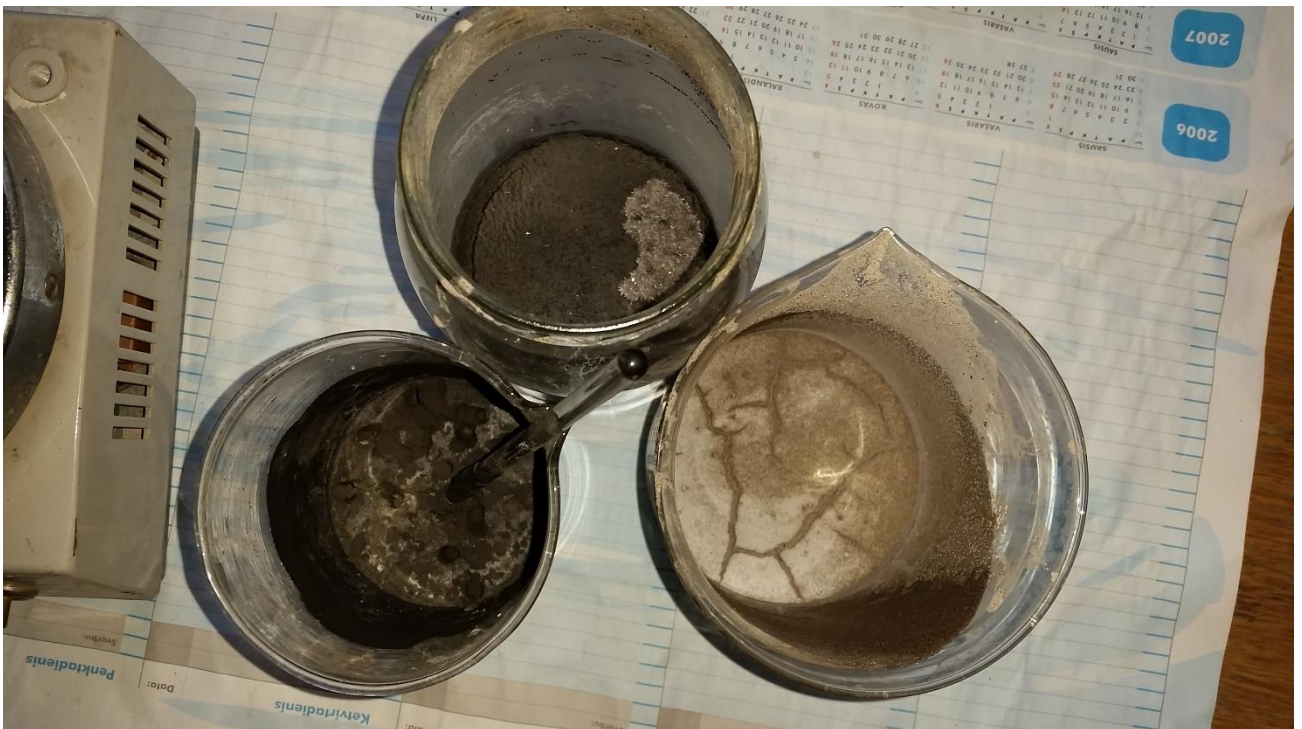
Figure 17. Type 1, Type 2, Type 3 BBA after chemical treatment and drying at 60 °C temperature
