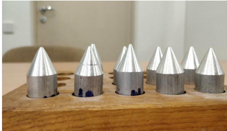
Fig. 3.2. Conical shape workpieces after machining
