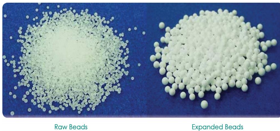
Figure 12 It Show the Raw Beads of Eps & Expanded Beads “Insulation Corporation of America”
