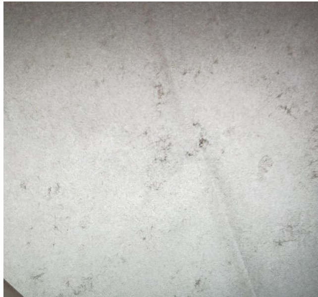
Fig.3.2. Polyethylene cover after removal of paper 10cm × 10cm
