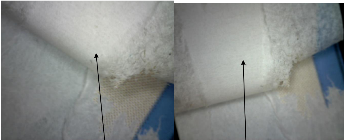
Figure.4.8. Failure mode of Cohesive.
