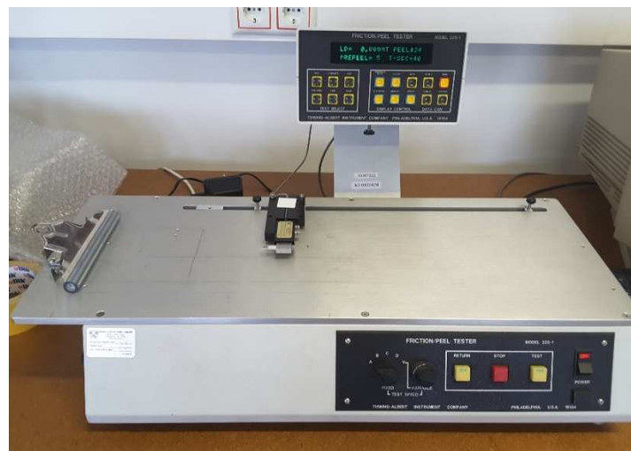
Figure 7. 5 Peel equipment used in the experiment
