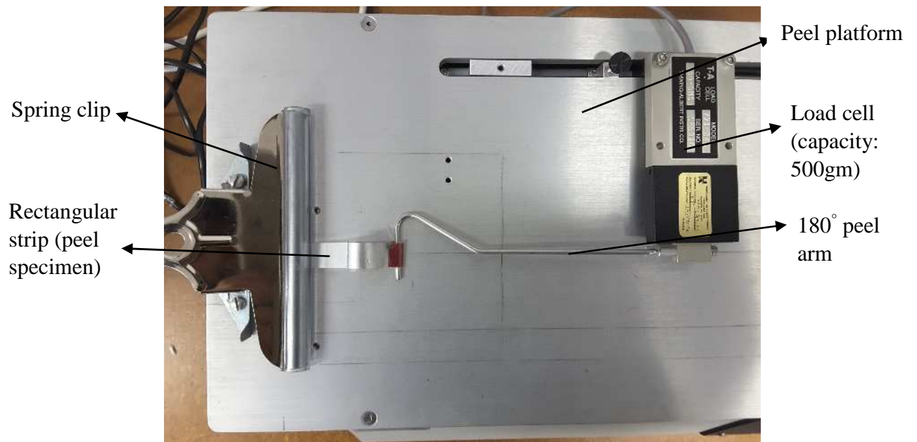
Figure 7. 7 View of peel test equipment and the apparatus
