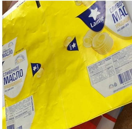
Figure 6. 2 Picture and structural view of foil laminated by paper and polyethylene
