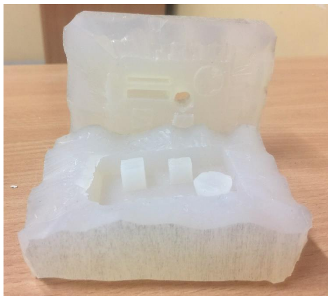
Fig.3.2.1 RTV 3428 silicon mould
