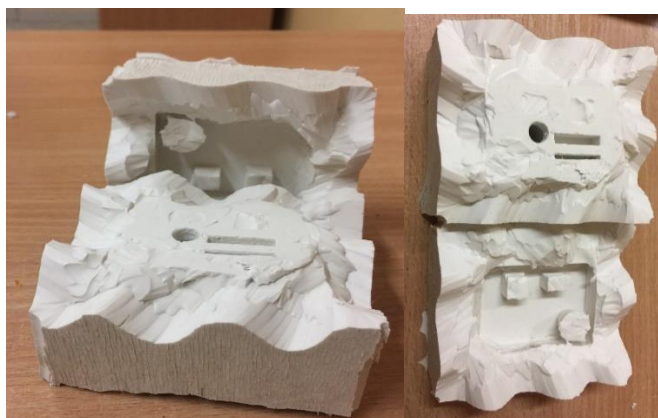
Fig.3.2.4 CENUSIL M 380 Silicone Mould
