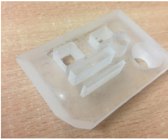
Fig 3.4.4 casted part by polyurethane
