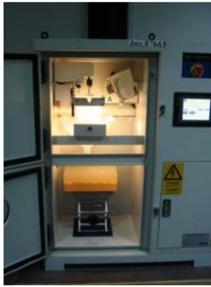
Fig.2.2 MCP-001P Vacuum Casting Machine [5]
