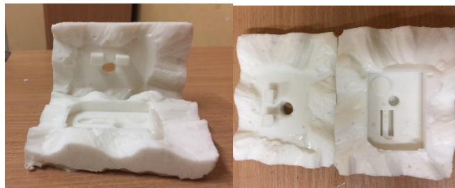
Fig. 3.2.10 KDSV THX-30 silicone mould
