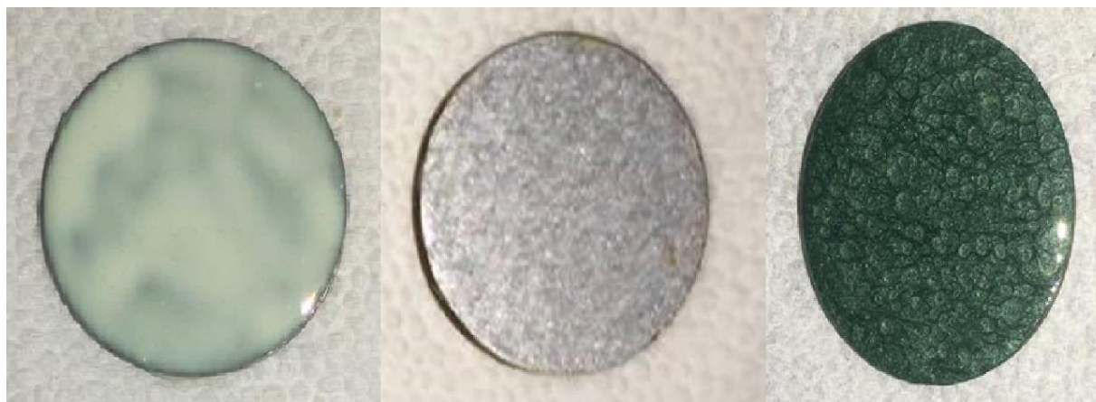
Fig. 2.4. Application of Ferox and anti-corrosive paints
