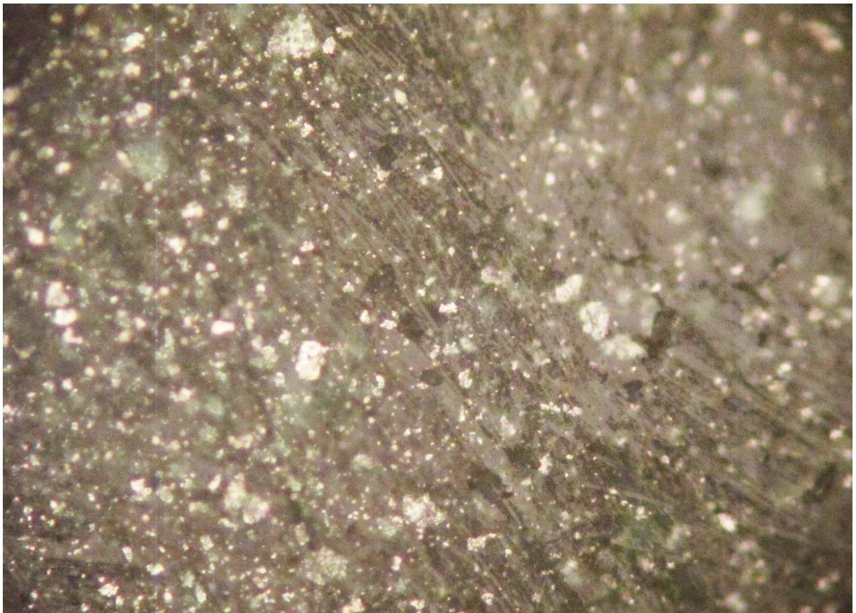
Image: 9222 Penta color after passivation test. Magnification = 20x
