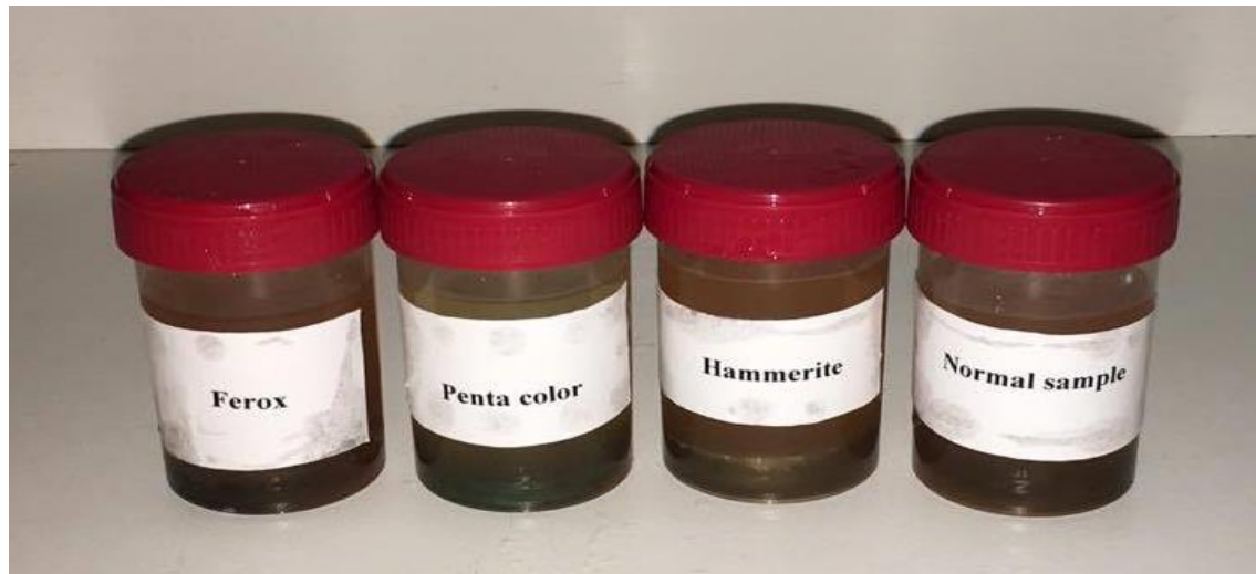
Fig. 2.5. Initial step of salt spray test
