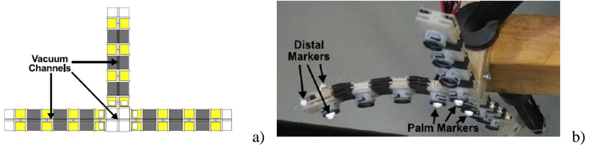
Figure 4: The three-fingered gripper : a) representation of the three-fingered gripper ; b) experimental setup [13]
