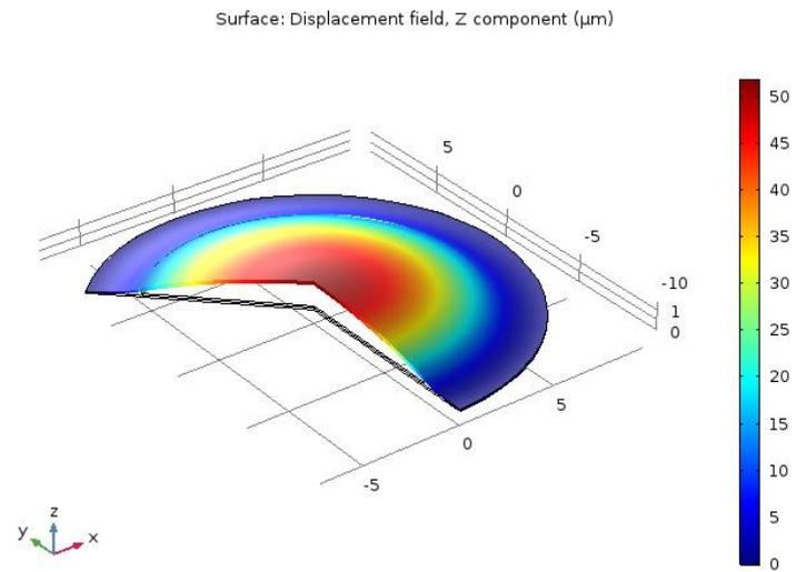
Figure 27: The displacement of brass membrane actuated by PZT ( 90V )
