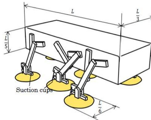
Figure 8: Schematic of the robot model and the locomotion mechanism [17]
