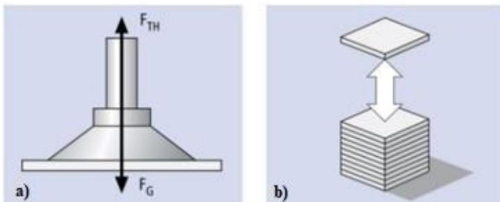
Figure 30: Schematic representation a) of forces acting on horizontal lifting; b) direction of work material movement.
