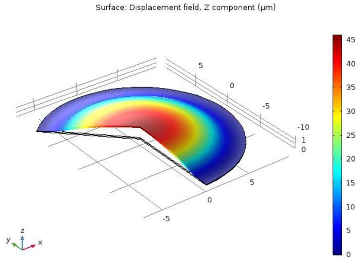
Figure 26: The displacement of brass membrane actuated by PZT ( 80V )
