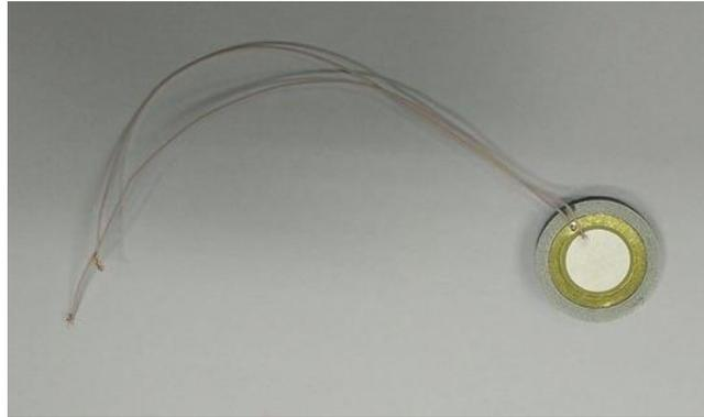
Figure 32: Brass membrane attached to PZT, fixed to plastic frame
