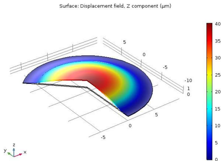
Figure 25: The displacement of brass membrane actuated by PZT ( 70V )
