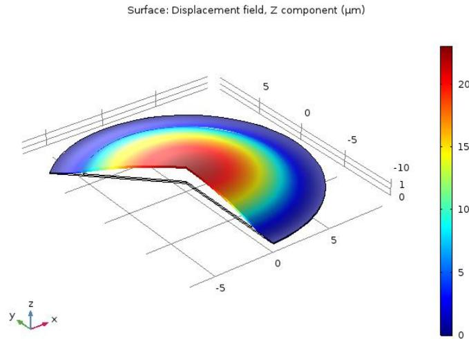
Figure 22: The displacement of brass membrane actuated by PZT ( 40V )
