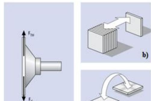
Figure 29: Schematic representation a) forces acting on vertical lifting; b) and c) direction of work material movement.
