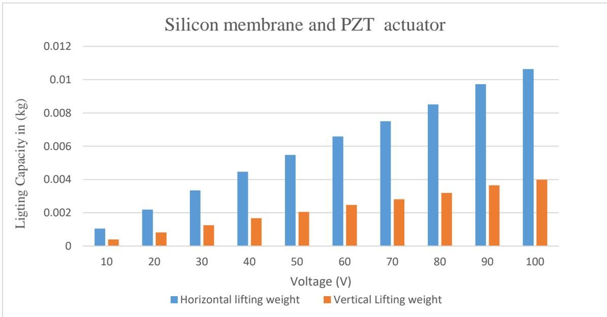
Graph 8: Dependency of lifting capacity with the applied voltage for silicon membrane actuated using PZT
