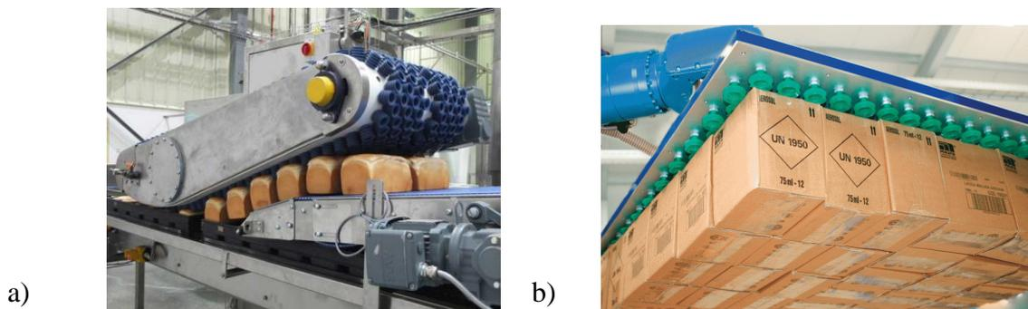
Figure 34: Industrial applications of suction cup: a) array of suction cups used in food industry; b) packaging industry [32]
