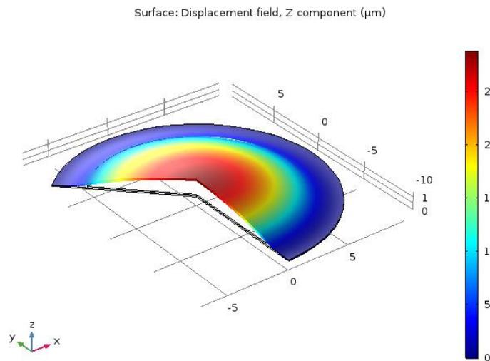
Figure 23: The displacement of brass membrane actuated by PZT ( 50V )
