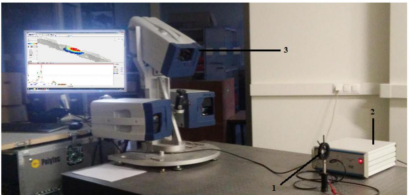
Figure 31: Experimental setup: 1) brass membrane with piezoelectric actuator; 2) linear amplifier P200 (FLC Electronics AB, Sweden), 3) 3D scanning vibrometer PSV-500-3D-HV (Polytec GmbH, Germany)
