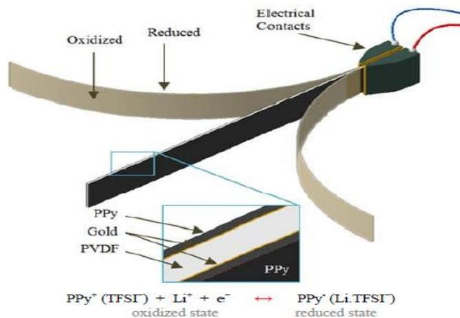
Figure 5: Structure and operation of EAP actuator [14]
