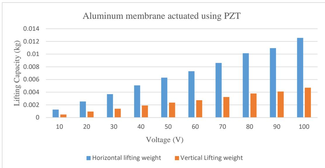
Graph 5: Dependency of lifting capacity with the applied voltage for aluminum membrane actuated using PZT
