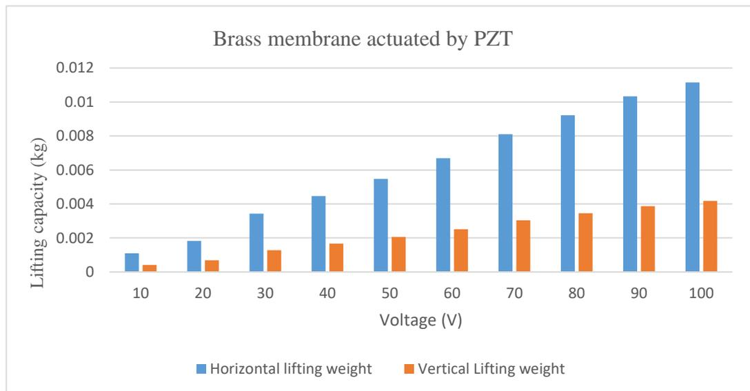
Graph 7: Dependency of lifting capacity with the applied voltage for brass membrane actuated using PZT
