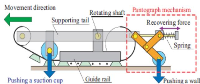
Figure 11: Suction cup working mechanism [20]
