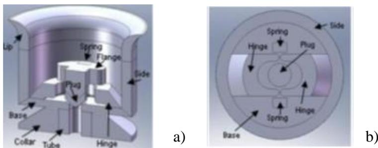
Figure 2: Cross section of suction cup: a) cross sectional view; b) top view [12]
