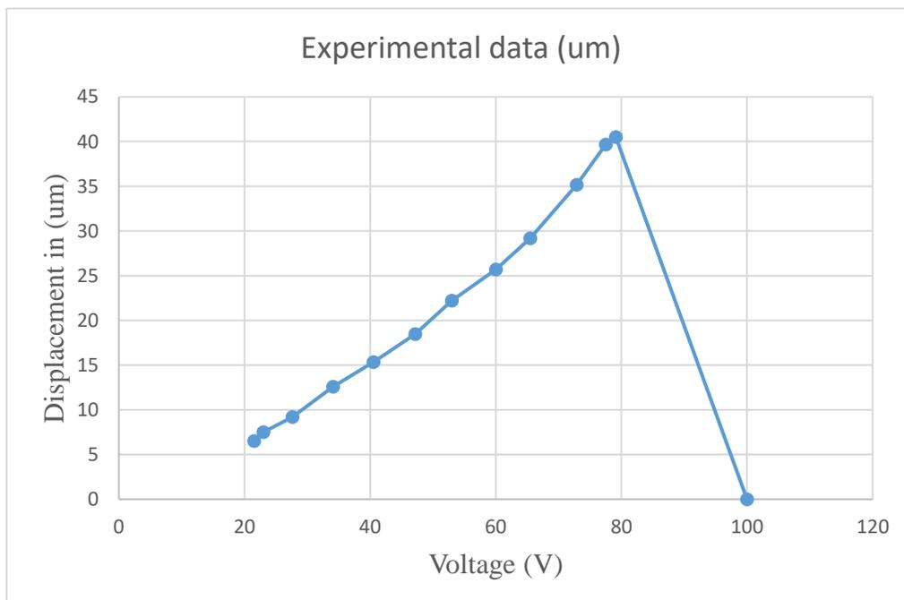
Graph 9: Experimental data of brass membrane actuated using PZT
