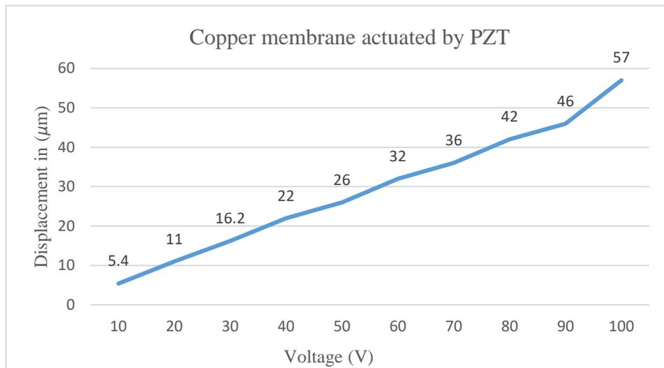
Graph 3: Relationship between the displacement and voltage for copper membrane actuated by PZT
