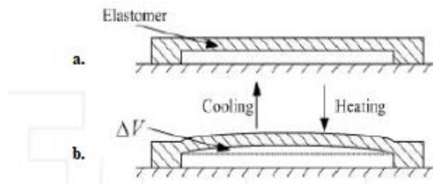
Figure 1: The sealed air cavity in the elastic material: a) before activation; b) after activation [9]
