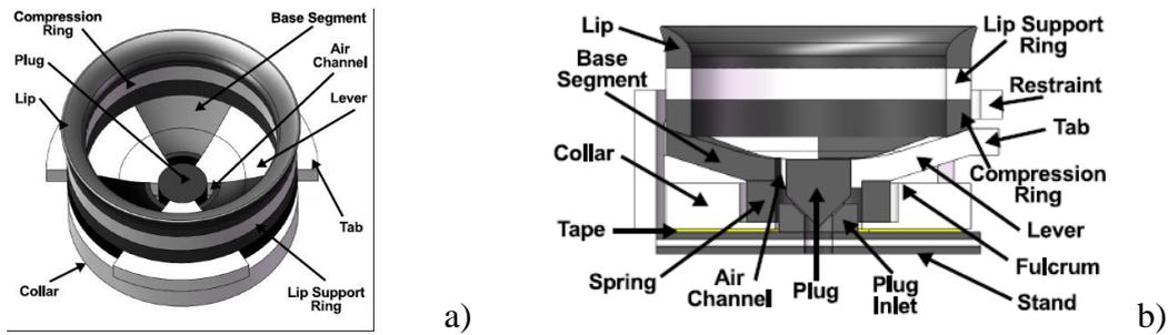
Figure 3: Schematic of self-healing cup : a) top view; b) cross sectional view [13]
