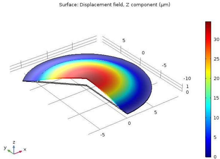
Figure 24: The displacement of brass membrane actuated by PZT ( 60V )
