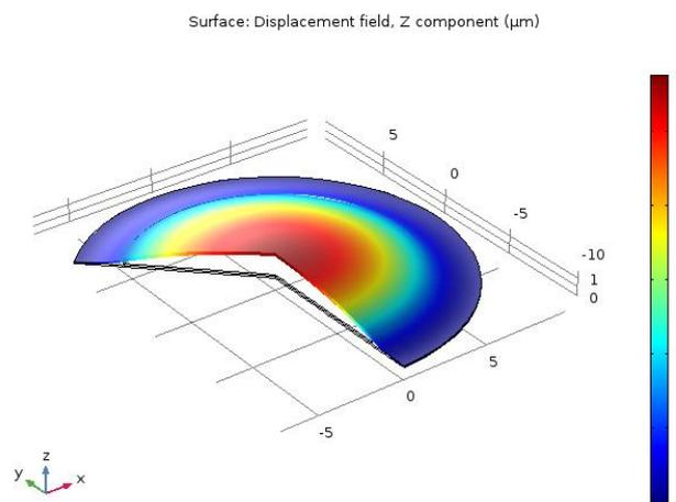
Figure 19: The displacement of brass membrane actuated by PZT ( 10V )
