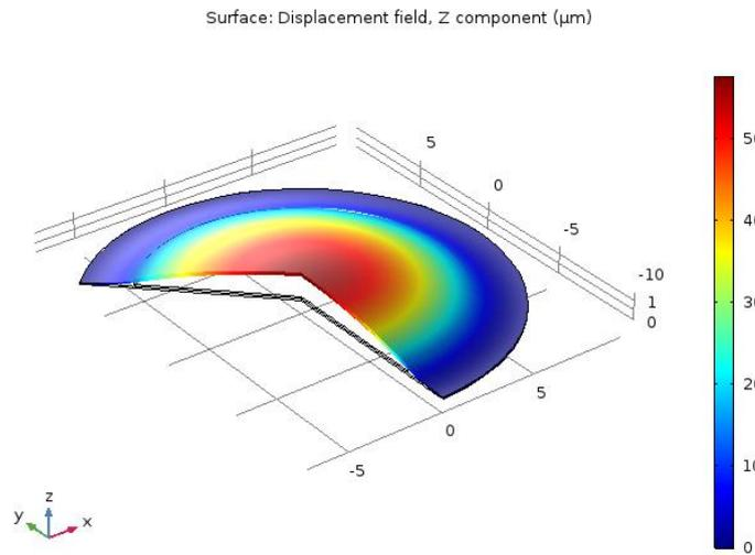
Figure 28: The displacement of brass membrane actuated by PZT ( 100V)
