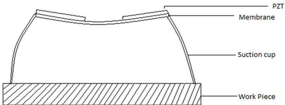
Figure 17: 2D representation of the suction cup with negative displacement
