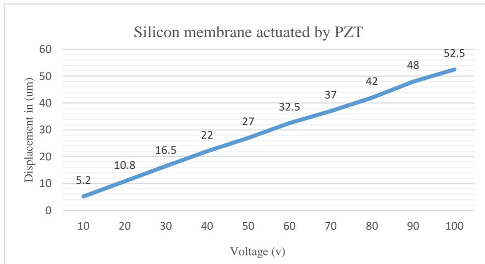
Graph 4: Relationship between the displacement and voltage for silicon membrane actuated by PZT
