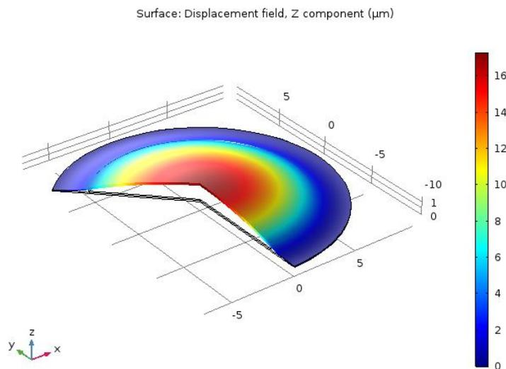
Figure 21: The displacement of brass membrane actuated by PZT ( 30V )
