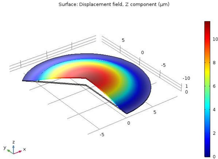
Figure 20: The displacement of brass membrane actuated by PZT ( 20V )
