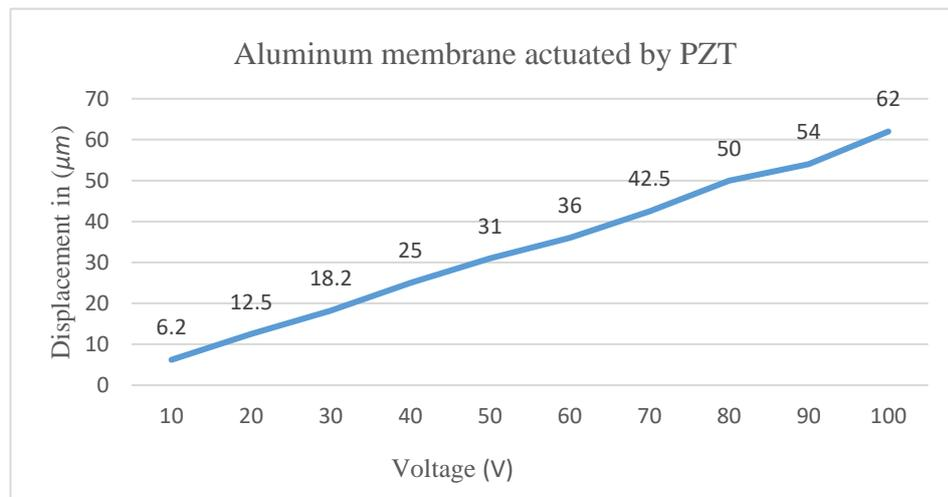
Graph 2: : Relationship between the displacement and voltage for aluminum membrane actuated by PZT
