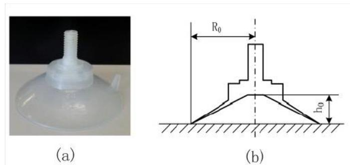
Figure 14: Suction cup a) commercially available; b) cross sectional view [22]
