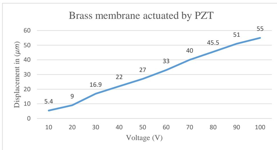
Graph 1: Relationship between the displacement and voltage for brass membrane actuated by PZT
