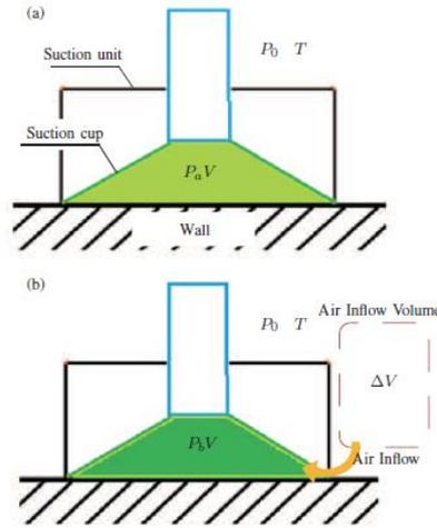
Figure 6: Analysis of air in flow a) initial status of suction cup attached to the surface (b)changing status of suction cup inner pressure [15]
