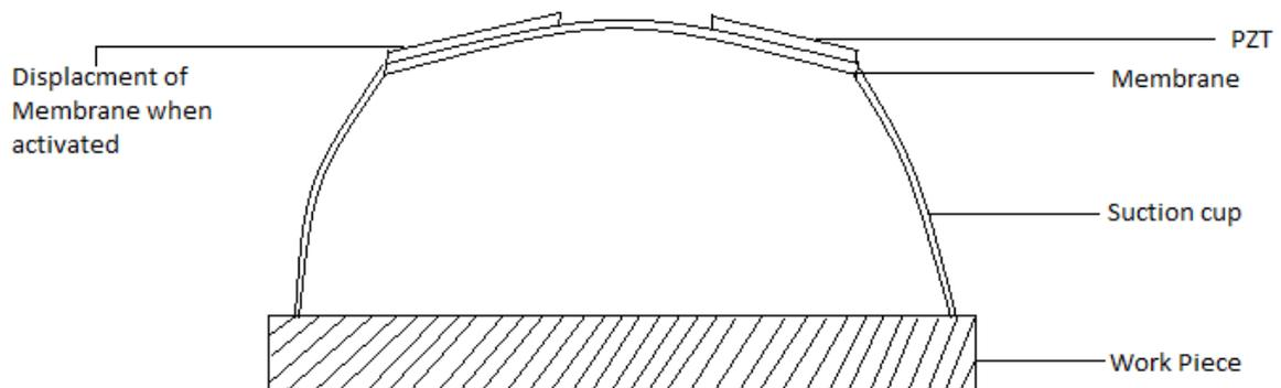
Figure 18: 2D representation of the suction cup with postive displacement
