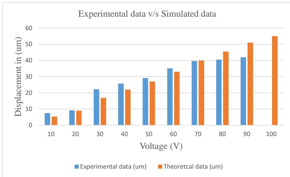
Graph 10: Experimental data v/s simulated data for brass membrane actuated by PZT
