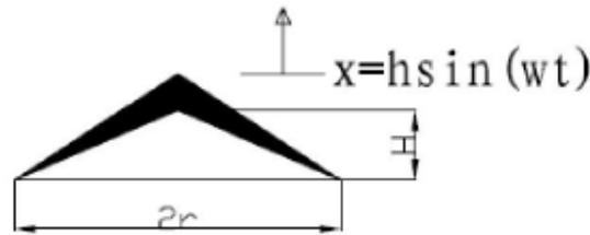
Figure 12: A vibration cycle of the suction and the conical figure of the cup [21]
