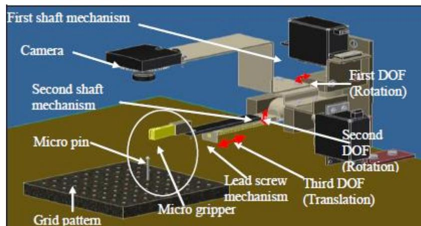
Figure 7: CAD model of piezo actuator based micro manipulation system. [16]
