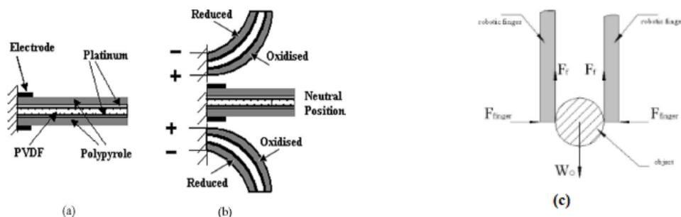
Figure 9: Schematic structure :a) conducting polymer actuator; b) representation of the bending principle; c) gripper handling a spherical object [18]
