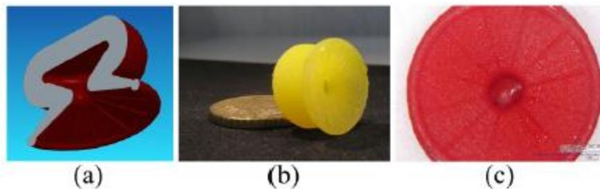
Figure 10: CAD model of the sucker: a) cross sectional view; b) 3D printed ; c) bottom view [19]
