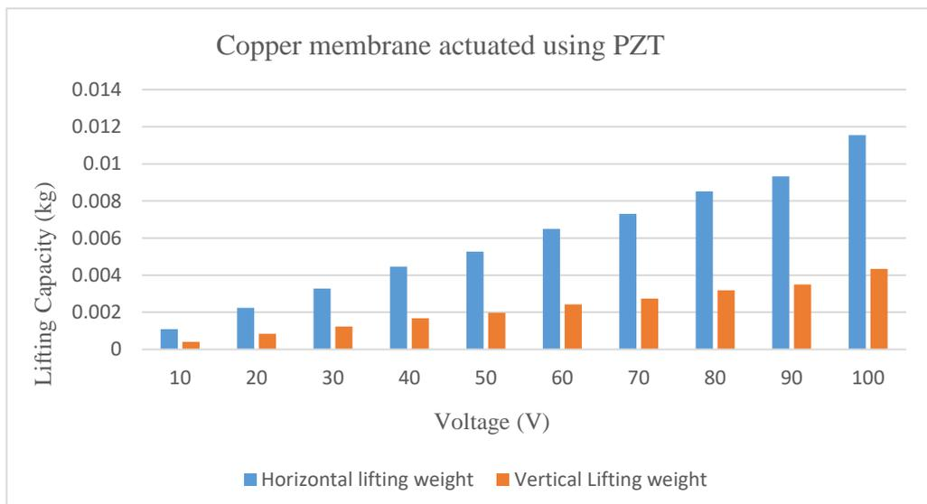
Graph 6: Dependence of lifting capacity with the applied voltage for copper membrane actuated using PZT
