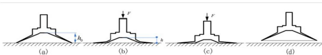
Figure 13: Working phases: a) initial phase; b) pushing phase; c) attached phase; d) detached phase [22]
