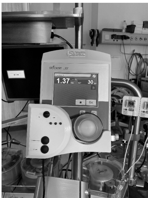
Figure 2.—The mechatronic plug-in device BrainProtect used during the clinical trial for implementing a novel mode of HLM (Stöckert S5) operation – rectangular modulation of blood flow for real-time CA status monitoring and blood flow control during the CPB.
