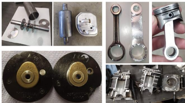
Fig 8. Modifications made to the engine. Top left – custom exhaust vs stock GX35. Top right – GX35 stock con rod vs custom. Bottom left – stock camshaft vs machined. Bottom right – GX35 cut open for examination.
