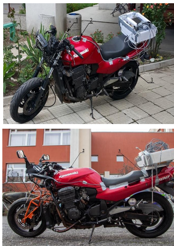
Fig.2. Kawasaki motorcycle equipped measuring equipment, 1-front suspension sensor, 2- accelerometer, 3 rear suspension displacement sensor
