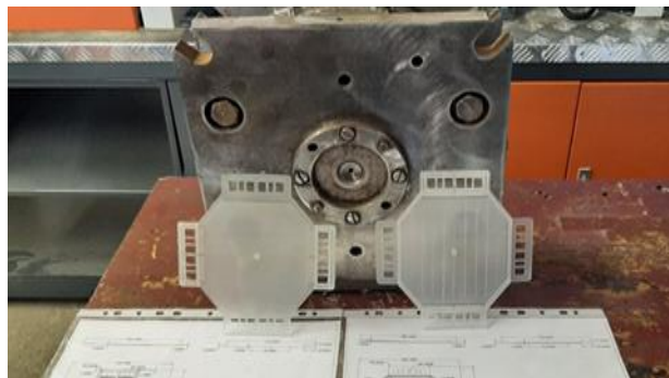
Fig. 4 Filter-drainage and turbulator, casting mold and molded plastic parts
