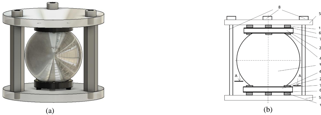
Fig.6. Spherical magnetic drive: a – model view; b – schematic view: 1-elastic supports; 2 – resistant-free support; 3-magnetic sphere; 4- piezoelectric transducers; 5 – flanges; 6 – sides of continuous electrodes of piezoelectric rings; 7 - sides of divided electrodes of piezoelectric rings; 8 – bolts.
