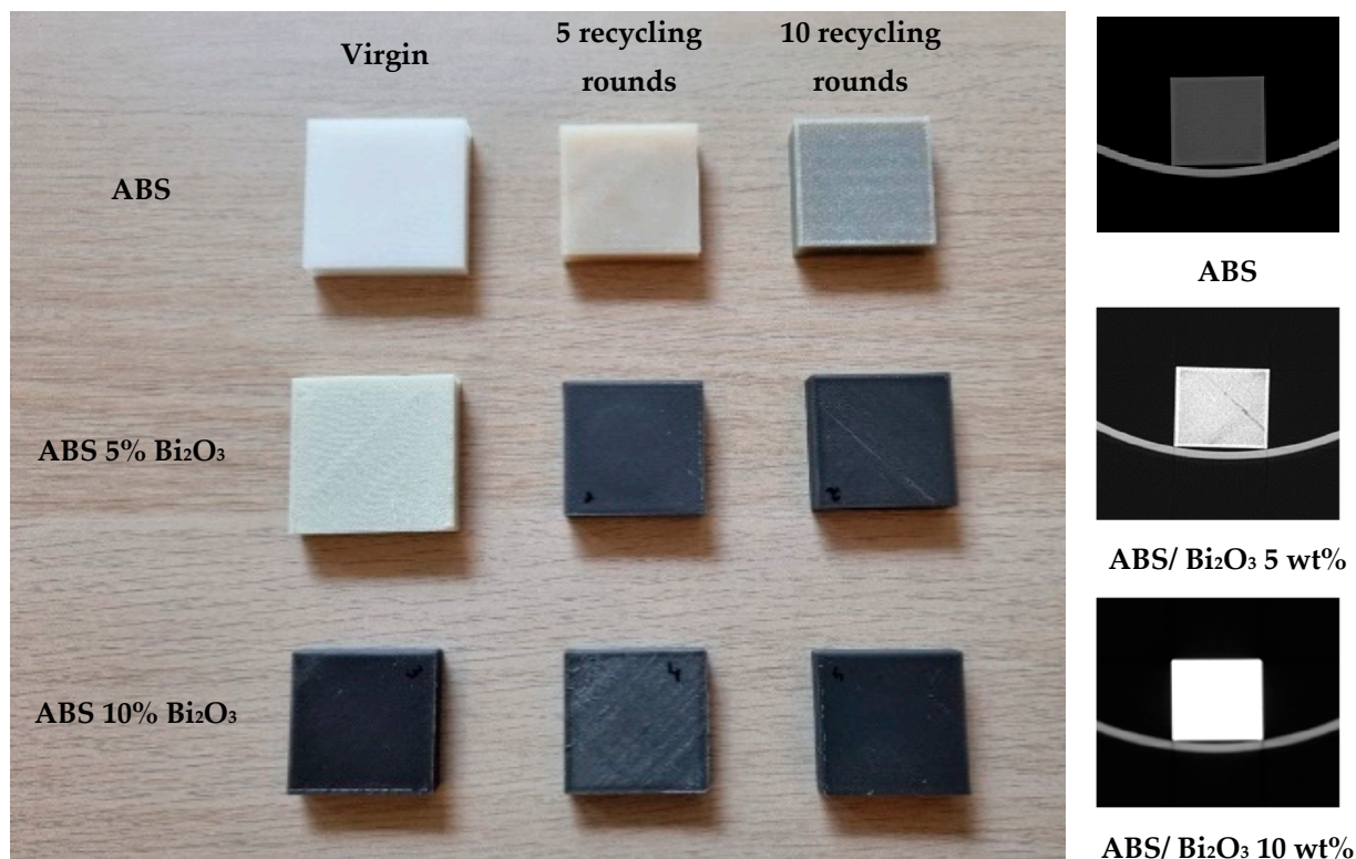
Figure 2. Visual appearance of 3D-printed samples after various recycling rounds (Left) and CT scans of virgin samples (Right).
