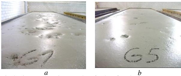
Fig. 2. The optical microscopy micrographs of cake after the intense outgassing of H_2 when the amount of cement were, %: a – 13.7; b – 23.6.
