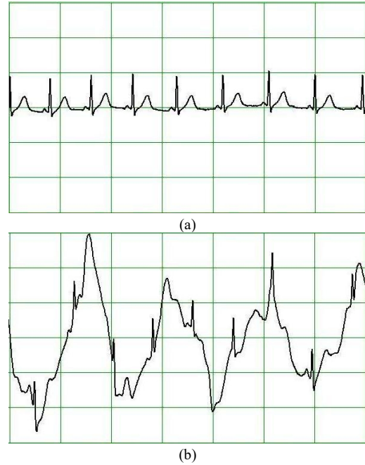
Fig. 6. ECG signal during rest (a) and torso rotation (b). Time scale is 1 s/div.
