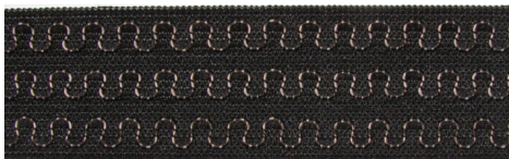
Fig. 2. Fragment of inductive sensor with 3 parallel coils interwoven into expandable belt sewn into T-shirt.
