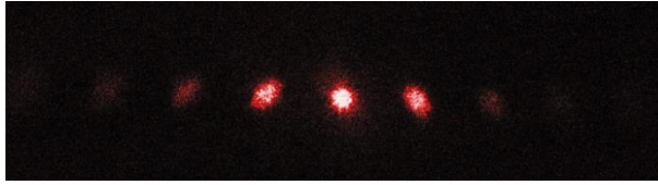
Fig. 4.17. Transmitted diffraction pattern generated due to the interaction of He-Ne laser light with the polymeric scale
