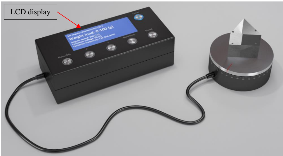
Fig. 5.3. A geometric virtual model of the proposed prototype of high-resolution piezoelectric rotary stage: a) an overall view; b) the stage in action (positioning of optical element)
