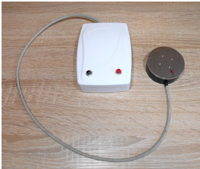
Fig. 5.5. The physical prototype of a high-resolution piezoelectric rotary stage with an integrated closed-loop feedback control system
