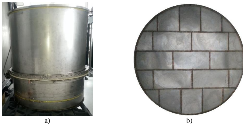
Fig. 5.2.2. The mock-up of the scaled-down storage tank (a) and the construction of the storage tank floor (b)
