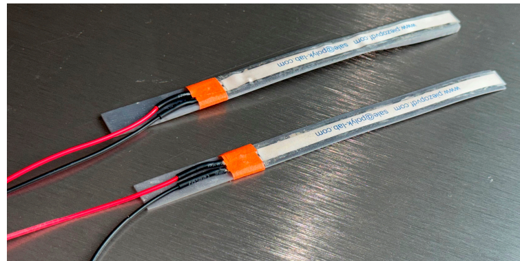
Figure 11. Illustration of the manufactured cantilevers—top cantilever is optimal shape and bottom cantilever is uniform shape.
