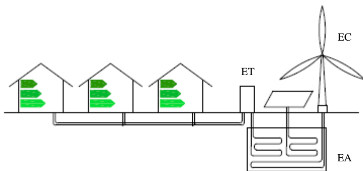
Figure 3.8. Wind energy conversion system for a group of consumers: Wind rotor – Heat generator (energy conversion EC) – Heat accumulator (energy accumulation EA) – Heat network of the locality – Heat pump (energy transformation ET) – Heating system of the building
