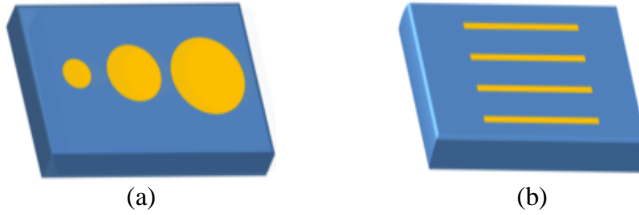
Fig. 62. Geometries of the electrode: (a) circular; (b) stripe electrodes
